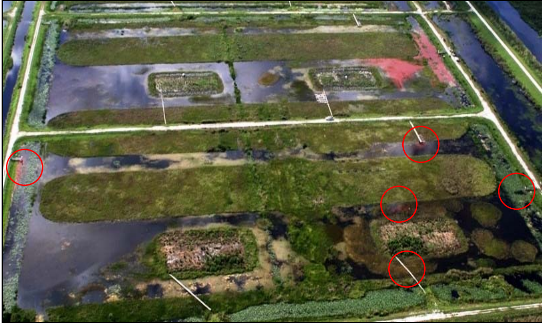
Figure 6.2.5.4. Comparison between flowing M2 (top of picture) and non-flowing M1 (lower), 1 hour after dye release.
