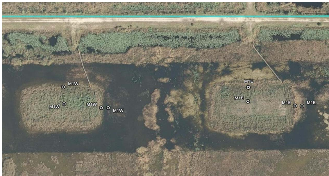
Figure 8.7. Georectified locations of SETs using M1 tree islands as an example. One SET is located on the “wet” side slope (upper in figure) and one is located on the highest elevation area of each tree island in the highest density plantings. Two other SETs are located in line with the tree island center at midslope and on the slough bottom of tree island tails.
